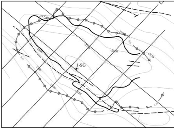
**Figure 1** Structural map of reflecting horizon I<sub>A</sub> with results of comparison of a water-oil contact' contour and IP anomaly contour by the DNME data. Legend: 1 - OWC contour; 2 - faults; 3 - IP anomaly contour.
