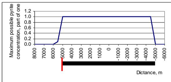
**Figure 5** Modelling of pyrite concentration for Severo-Gulyaevskaya subsurface model taking into account influence of a vertical fault (red).
