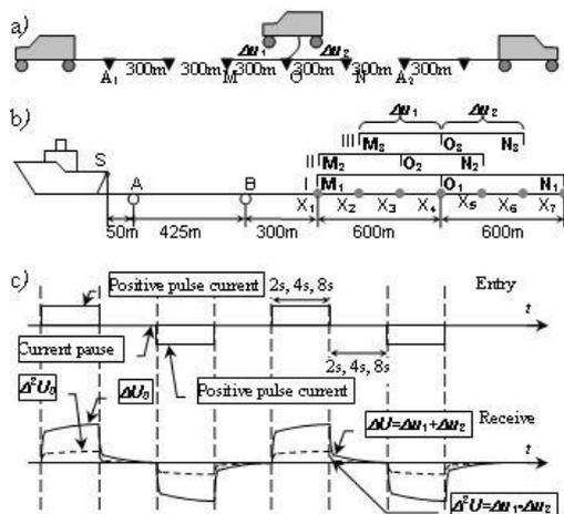
**Figure 1** The principles of the DNME method a) Land A1B1-MON-A2B2 setup with opposite power dipoles position b) Marine AB-MN setup with three offsets – I, II и III c) Electrical current profile in time for entry electrodes and measured voltage pattern on ADC input.
