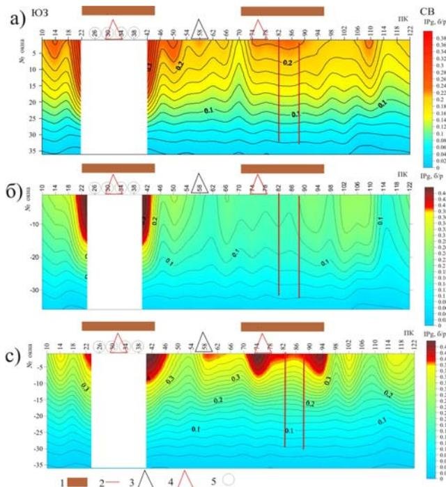
**Figure 5** Comparison of polarization fields IPg distribution at different time filters' usage: a)  $0.01 \text{ sec} \leq \tau \leq 5 \text{ sec}$ ; b)  $0.1 \text{ sec} \leq \tau \leq 5 \text{ sec}$ ; c)  $\tau < 0.1 \text{ sec}$  (1 – HC deposits confirmed by drilling; 2 – faults according seismics; 3 – empty wells; 4 – productive wells.
